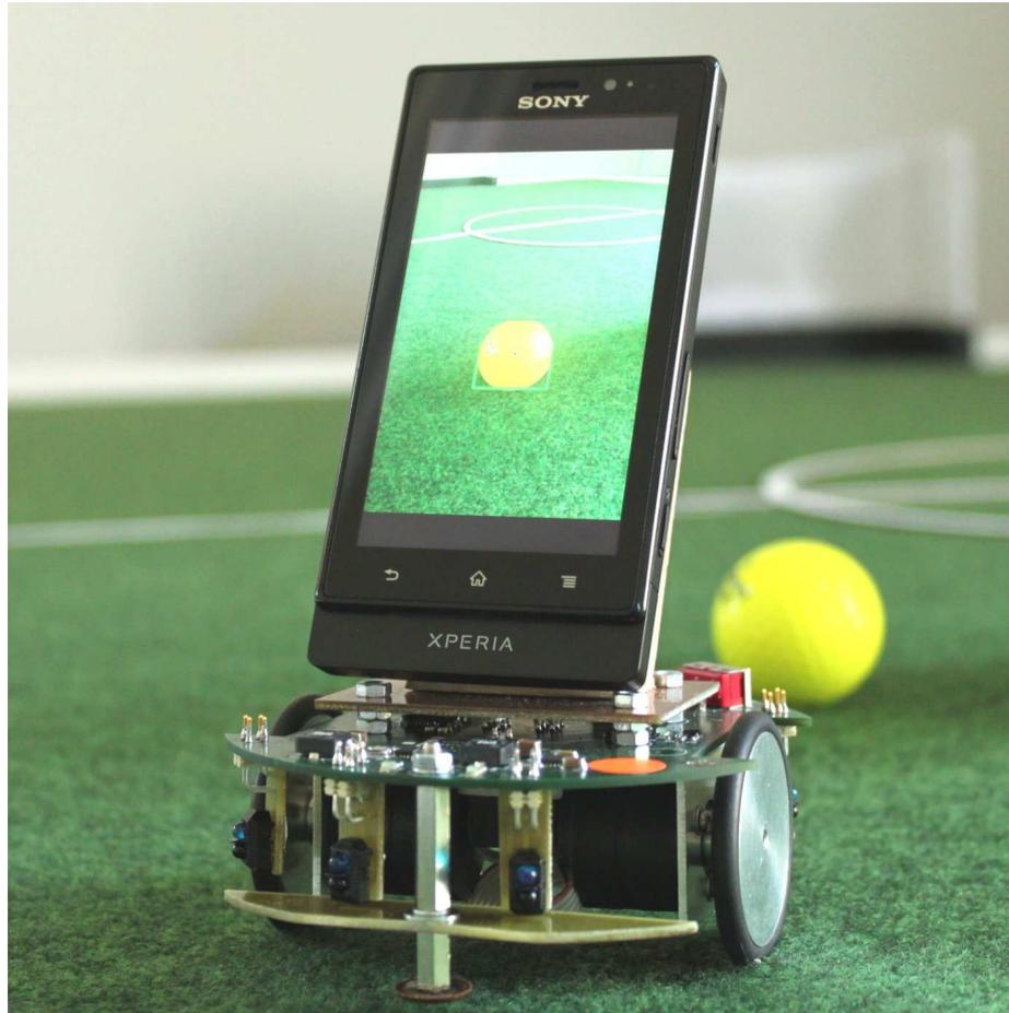
**Fig. 1.** Prototype for the mobile phone soccer robot
